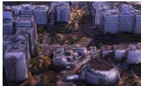
Figure 3: 3D model reconstructed using multi-view stereo.
