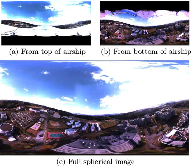
Figure 7: Full spherical HDR image generated from multi-exposure images captured by two omnidirectional cameras.
