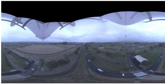
(a) A captured omnidirectional image. A missing area appear at top of the image.
