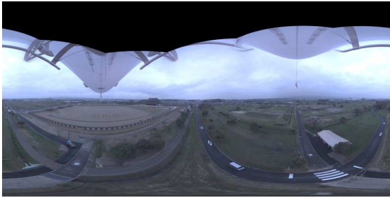
(a) An omnidirectional image aligned by the orientation of omnidirectional camera. A missing area appears at the top of the image.
