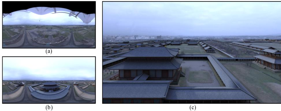
**Figure 1:** (a) An omnidirectional image aligned by the posture of omnidirectional camera. An invisible area appears at the top of the image. (b) An augmented omnidirectional image with virtual constructs superimposed using camera position and posture under the illumination environment of the real world. Invisible areas are inpainted from the input image. (c) A view-dependent perspective image converted from the omnidirectional augmented image in real-time.
