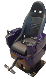
Figure 3: Motion base with two degrees of freedom.
